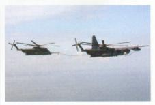
During the final 3 hour 55 min sortie, the MH-53Ms each took on board 250 lmp gal of fuel from a 352nd Special Operations Group MC-130P Hercules, which trailed drogues from its two underwing refuelling pods.
